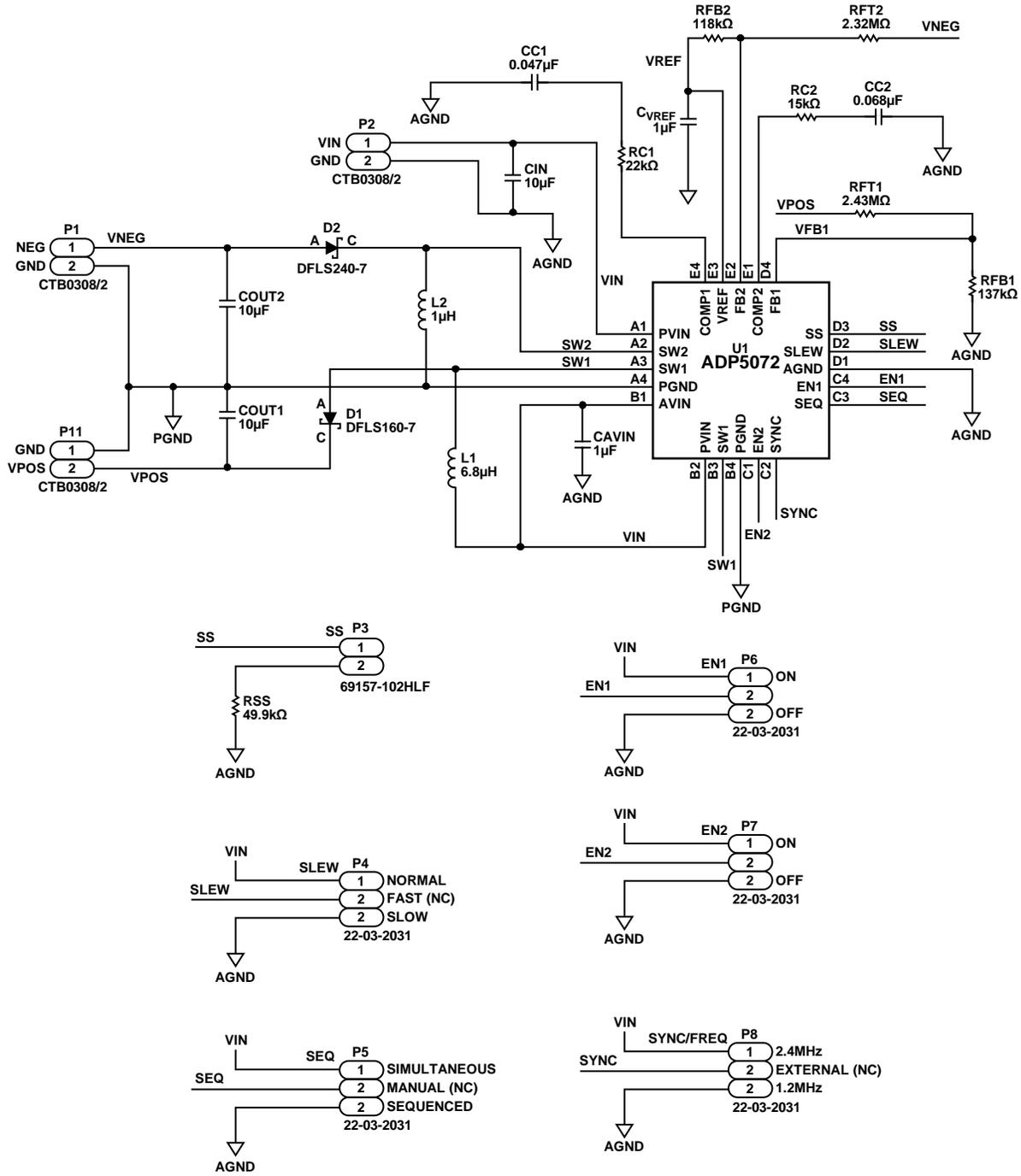
Figure 9. Evaluation Board Schematic for the ADP5072CB-EVALZ
