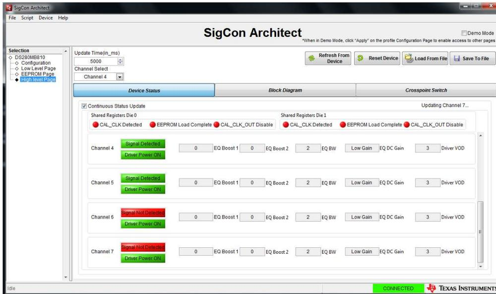
**Figure 7. SigCon Architect High Level Page: Device Status.**
