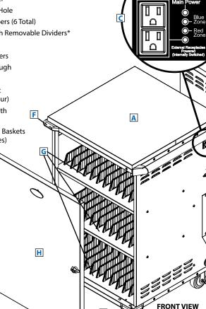
Locking steel cabinet wth charging, secure storage and cord management for up to 36 Ultrabooks, tablets and other devices
