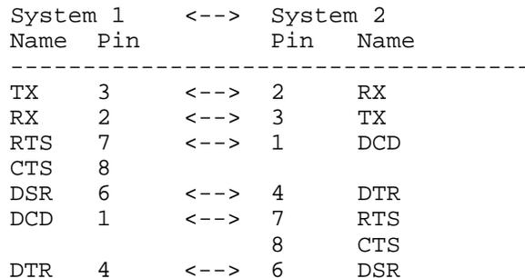
Pins 7 and 8 are shorted together on each connector. Unlisted pins have no connection.
