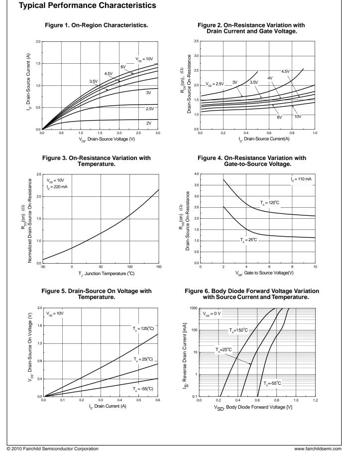
**BSS138W** — N-Channel Logic Level Enhancement Mode Field Effect Transistor
