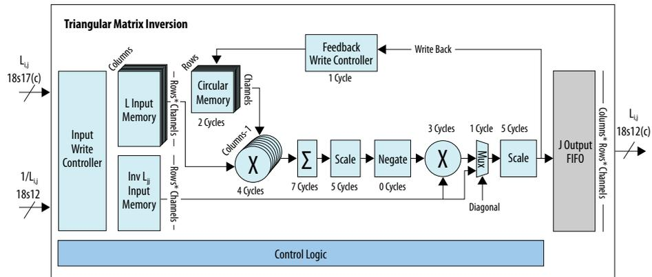
This design supports single-precision floating-point Cholesky matrix inversion. DSP Builder requires a single-precision floating-point input for the floating point inversion.
