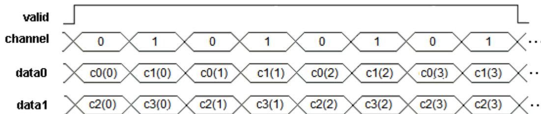
The channel signal remains a single wire, not a wire for each data wire. It counts over 0 to `ChanCycleCount - 1`.
