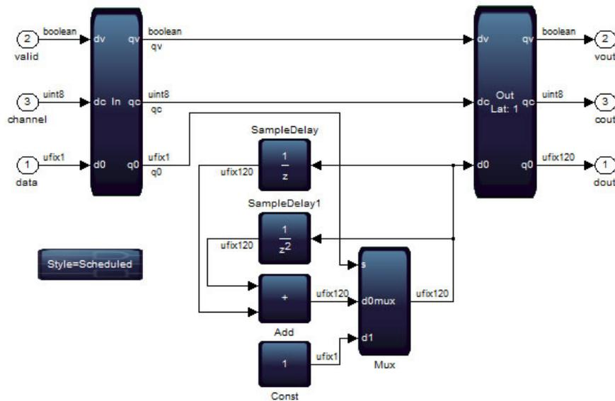
9. Select both of the **SampleDelay** blocks and point to **Rotate and Flip** on the popup menu and click **Flip Block** to reverse the direction of the blocks.
