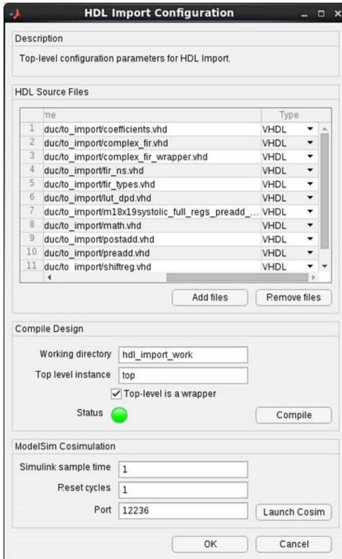
3. Add a **HDL Import** block to the digital\_up\_converter subsystem.
