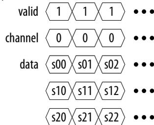
**Figure 6. Single Channel  $n > M$**
