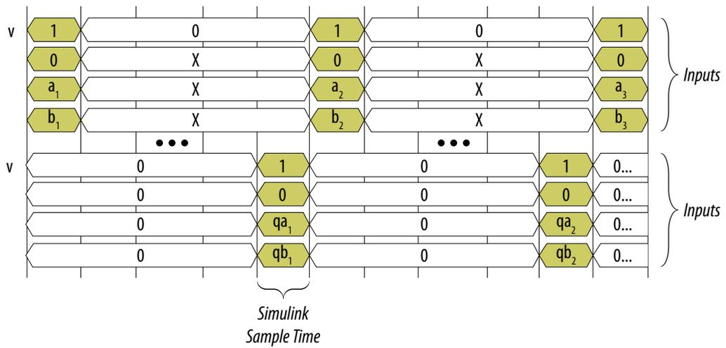
**Figure 84. Single Channel Clock Rate Simulation with Register Outputs**
