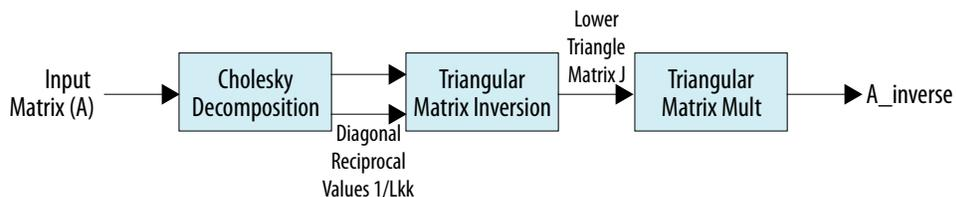
The Cholesky decomposition calculates the reciprocal values of the diagonal elements of  $L$ ,  $\frac{1}{L_{kk}}$  which the triangular matrix inversion requires. The design propagates those values to the output interface of the Cholesky decomposition reducing resource usage and latency.
