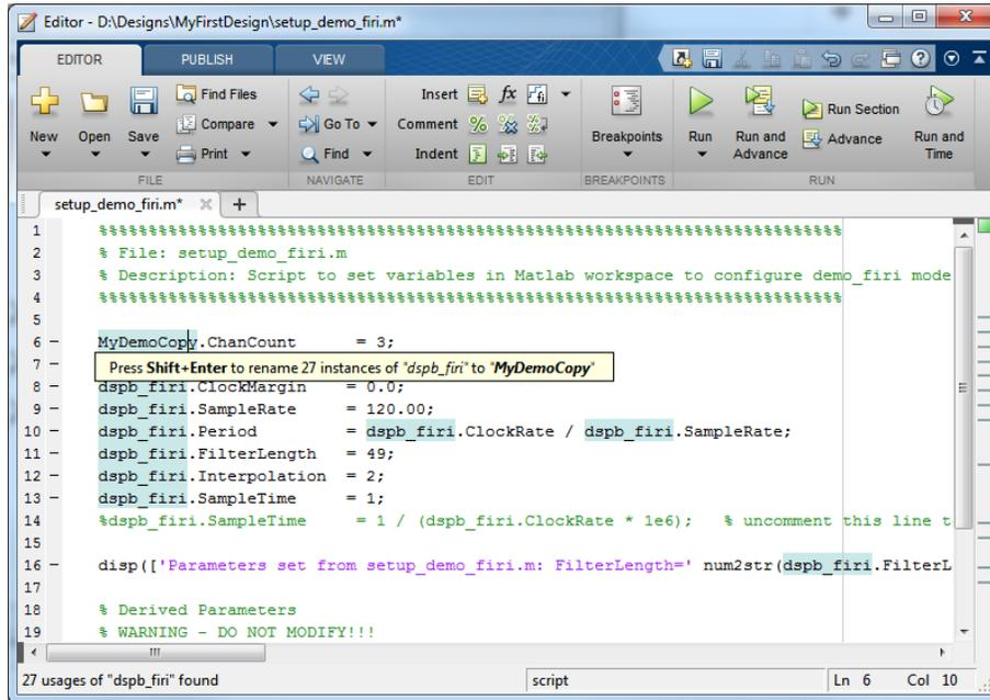
4. Open the new model file as text and globally replace the parameter structure to match.
