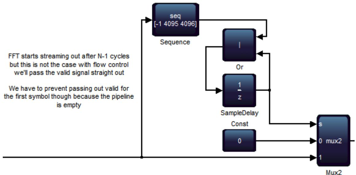
The latency that the **ChannelOut** block reports is therefore not 4096 + the automatic pipelining value, but just the pipelining value.
