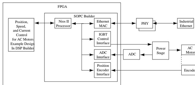
Each of the FOC, speed, and position feedback loops use a simple PI controller to reduce the steady state error to zero. In a real-world PI controller, you may also need to consider integrator windup and tune the PI gains appropriately. The feedback loops for the integral portion of the PI controllers are internal to the design.
