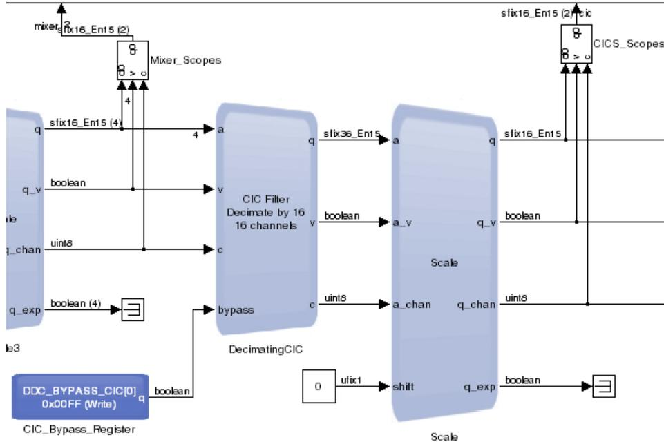
Two main blocks exist—the **DecimatingCIC** and the **Scale** block. To configure the CIC Filter, double click on the **DecimatingCIC** block.
