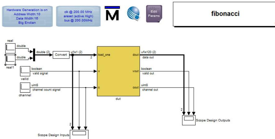
2. Copy the real input block, add a Simulink mux and connect to the Convert block.
