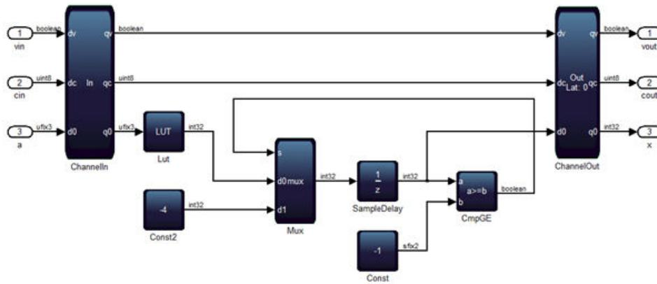
DSP Builder relocates the sample delay, to save registers, to the Boolean signal that drives the *s*-input of the 2-to-1 **Mux** block. You may see a mismatch in the first cycle and beyond, depending on the contents of the LUT.
