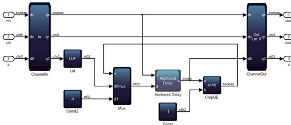
To make a control unit design resistant to automated delay redistribution and to solve most hardware FSM designs that fail to match simulation, replace every **SampleDelay** block with the **Anchored Delay** block from the **Control** folder in the Additional libraries. When the valid-in first goes high, the **Anchored Delay** block outputs one (or more) zeros, otherwise it behaves just like an ordinary **SampleDelay** block.
