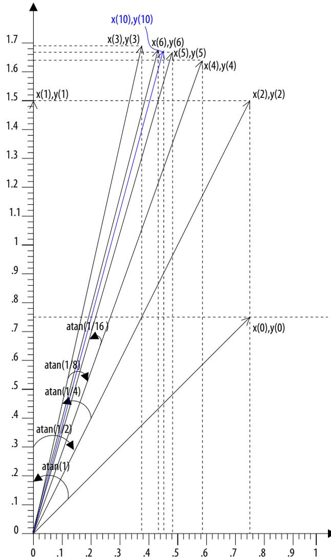
1. The input vector  $(x(0), y(0))$  is rotated to  $(x(1), y(1))$  by  $\text{atan}(1)=\pi/4$ .
