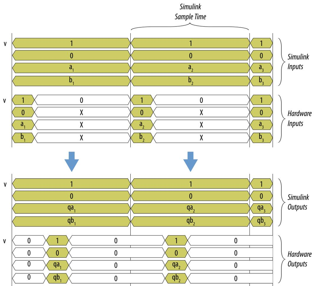
**Figure 82. Multichannel Data Rate Simulation with no Register Outputs**
