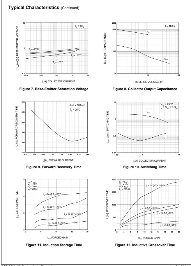
KSC5338D/KSC5338DW — NPN Triple Diffused Planar Silicon Transistor
