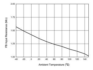
Figure 10. FB Input Resistance vs. Ambient Temperature
