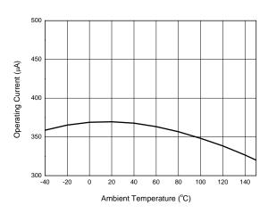
Figure 7. Operating Current vs. Ambient Temperature
