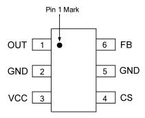
Figure 2. Pin Configuration of AP1686 (Top View)
