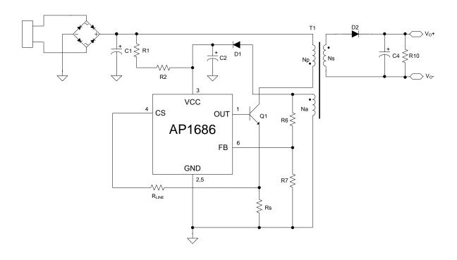
Figure 15. Typical LED Driver Application
