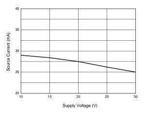
Figure 4. Operating Current vs. Supply Voltage
