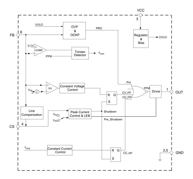
Figure 3. Functional Block Diagram of AP1686
