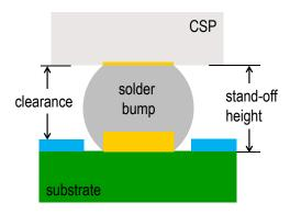
Figure 2 Collapsed solder bump after reflow.
