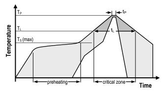
**Figure 1** Soldering profile according to JEDEC standard.  $T_P \le 260^{\circ}\text{C}$  and  $t_P \le 30\text{sec}$  for Pb-free assembly.  $T_L \le 220^{\circ}\text{C}$  and  $t_L \le 150\text{sec}$ . Ramp-up/down speeds shall be  $\le 5^{\circ}\text{C/sec}$ .
