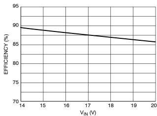
Figure 15. 12 V<sub>AC</sub> Input 5 W LED Driver Efficiency
