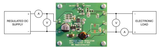
Figure 28. Test Setup for the NCP3065 Buck Evaluation Board
