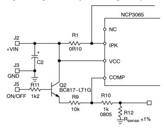
Figure 4. NCP3065 Dimming Solution A
