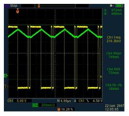
Figure 21. Switching Waveform Without Pulse Feedback
