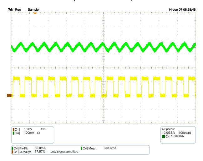
Figure 16. 12 V<sub>DC</sub>, I<sub>OUT</sub> = 350 mA Input Inductor Ripple Without Output Capacitor, C1 Inductor Input, C4 Inductor Current
