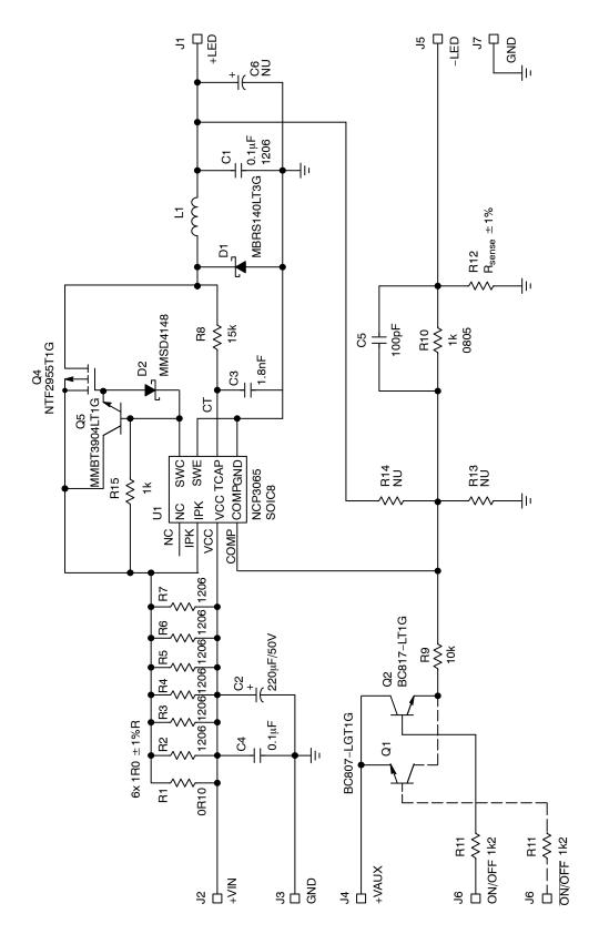
Figure 10. NCP3065 Buck Evaluation Board Schematic
