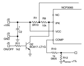
Figure 5. NCP3065 Dimming Solution B
