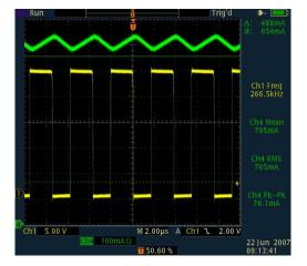
Figure 22. Switching Waveform With Pulse Feedback
