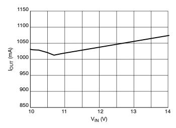
Figure 14. Current Regulation, 12 V<sub>DC</sub> Input 5 W LED Driver
