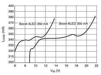
Figure 26. Line Regulation for 4 or 6 LEDs and Output Current 350 mA
