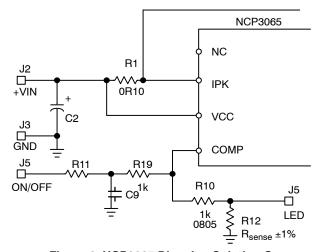
Figure 6. NCP3065 Dimming Solution C
