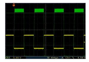
Figure 18. NCP3065 Dimming Behavior, Frequency 1 kHz, Duty Cycle 50%
