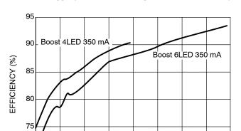
Figure 25. Boost Converter Efficiency for 4 or 6 LEDs and Output Current 350 mA
