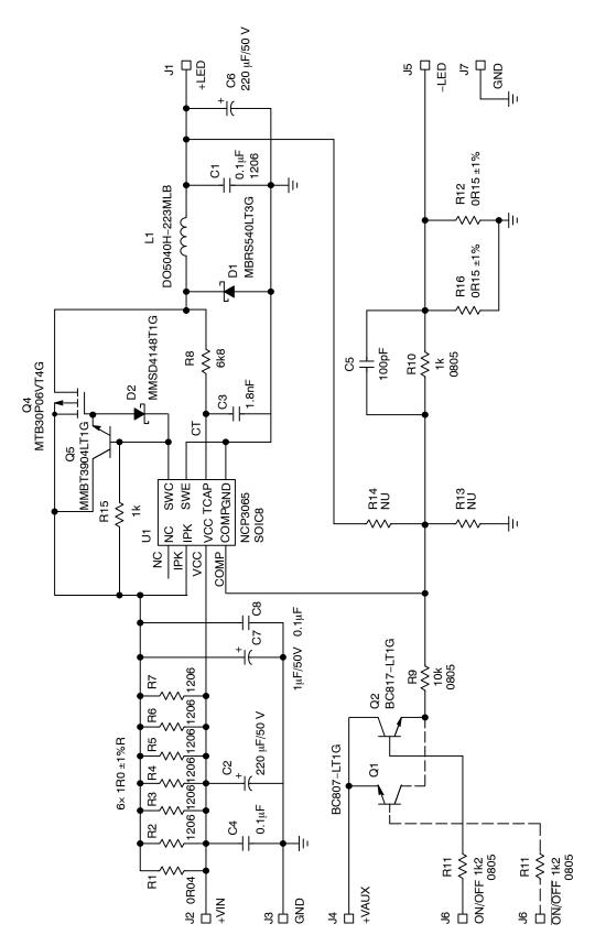
Figure 9. NCP3065 3A Buck Evaluation Board Schematic
