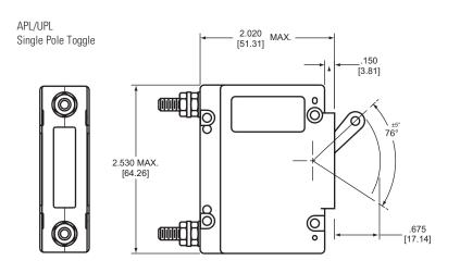
Note: Tolerance ± .015 [.38] unless noted. Dimensions in brackets [] are millimeters.
