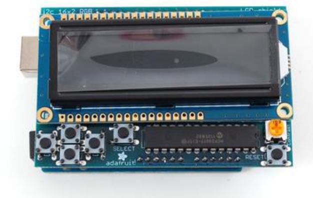
If your LCD does not have an RGB backlight or it has no backlight, you may have to shorten the length of header (see the previous step) until it matches and make sure the LCD fits over the silkscreen outline.
