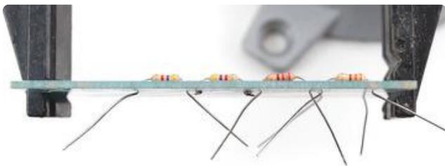
Make sure the resistors all sit nice and flat against the PCB.
