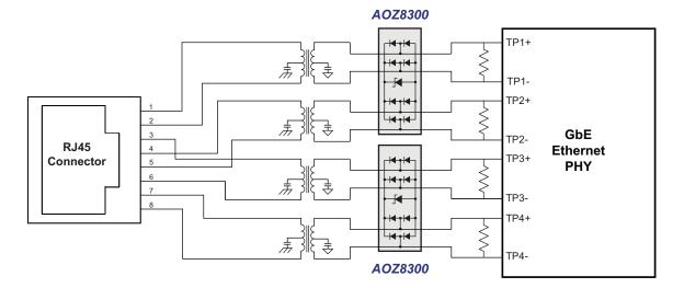
Figure 1. 10/100/1000 Ethernet Port Connection
